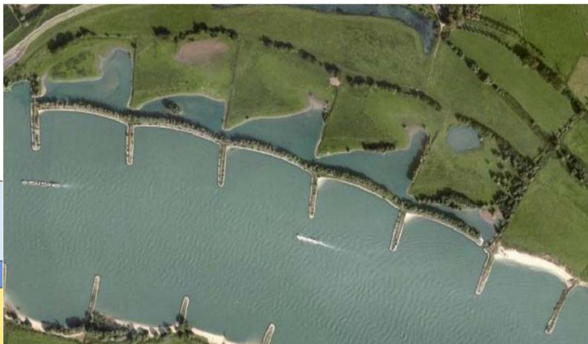
(Groins with off-bank protection Opijnen, The Netherlands)
